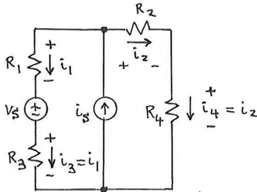
In the circuit diagram, only  $i$ 's are shown, with the understanding that  $v$ 's are given by Ohm's law:  $v = iR$ .
