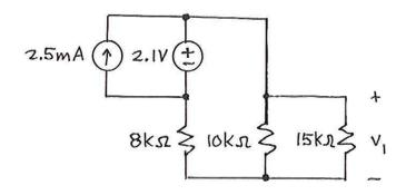
We see that the  $10k\Omega$  is in parallel with the  $15k\Omega$ .
