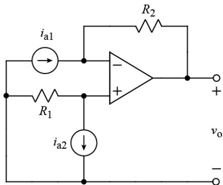
The op-amp operates in the linear mode. Using an appropriate model of the op-amp, derive an expression for  $v_o$  in terms of not more than  $i_{a1}$ ,  $i_{a2}$ ,  $R_1$ , and  $R_2$ .
