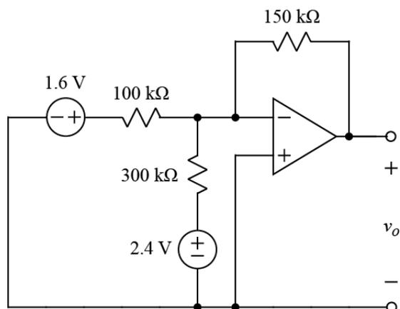
The op-amp operates in the linear mode. Using an appropriate model of the op-amp, find the value of  $v_o$ .
