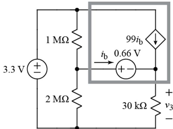
Find  $i_b$ ,  $v_3$ , and the power dissipated by the components in the box.
