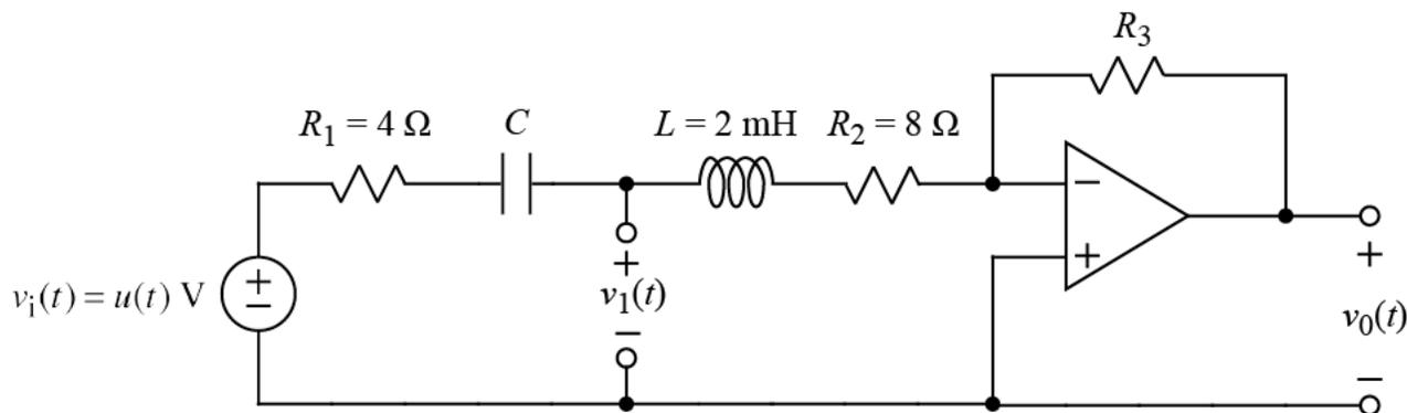
The voltage source in the above circuit is off (0 V) for  $t < 0$ .
