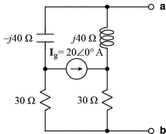
The impedance in the top half of the circuit is  $0 \Omega$ . Consequently, all the current from the current source will flow in the top half of the circuit, and no current will flow around the bottom half.
