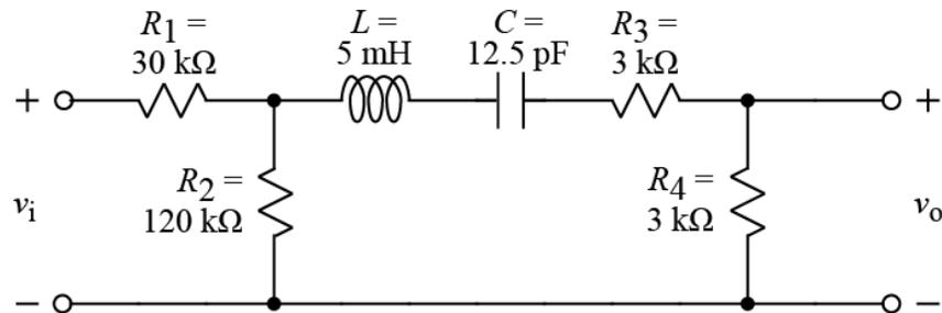
The above circuit is part of a simple crossover network for driving a midrange speaker having an impedance of  $8\Omega$ . The circuit is described at the following web site: <http://www.termpro.com/articles/xover2.html>. A more in-depth discussion of crossover networks may be found at <http://sound.westhost.com/lr-passive.htm>.
