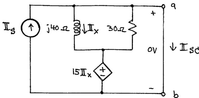
We observe that shorting  $a$  to  $b$  gives  $0V$  across the components in the middle. We suspect all of  $I_s$  flows in the wire from  $a$  to  $b$ , meaning  $I_x = 0$  and  $15I_x = 0V$ .
