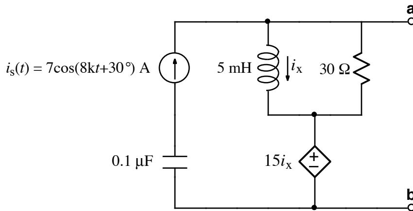
Draw a frequency-domain equivalent of the above circuit. Show a numerical phasor value for  $i_s(t)$ , and show numerical impedance values for R, L, and C. Label the dependent source appropriately.
