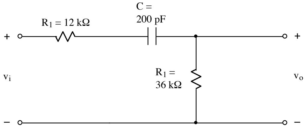
Note: vertical resistor should be labeled  $R_2$ .
