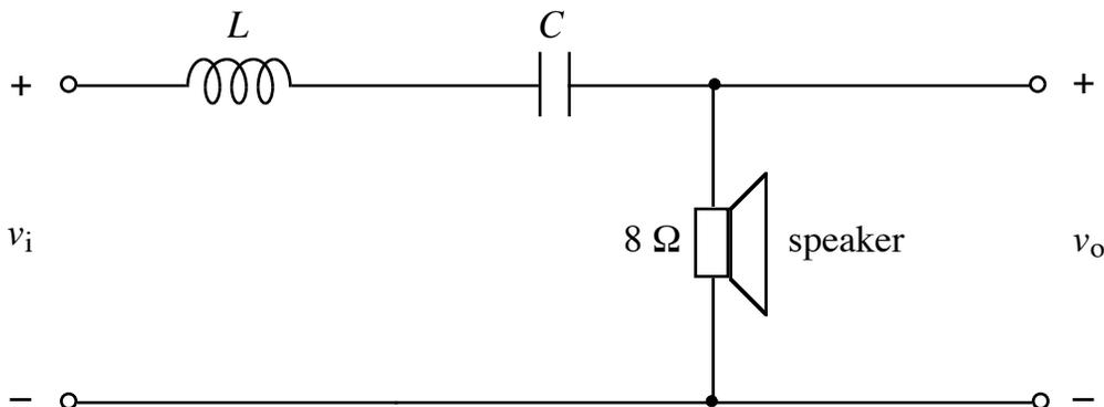
The above circuit is part of a simple crossover network for driving a midrange speaker having an impedance of  $8\Omega$ . The circuit is described at the following web site: <http://www.termpro.com/articles/xover2.html>. A more in-depth discussion of crossover networks may be found at <http://sound.westhost.com/lr-passive.htm>.
