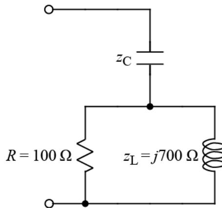
We compute the total impedance of the circuit and express it in  $a + jb$  form so that we can set the imaginary part, i.e.  $b$ , to zero.
