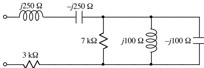
The series  $L$  and  $C$  in series at the top left of the circuit sum to zero, which means they cancel out to act like a wire. The parallel  $L$  and  $C$  at the right combine to create an equivalent impedance of infinity, or an open circuit.
