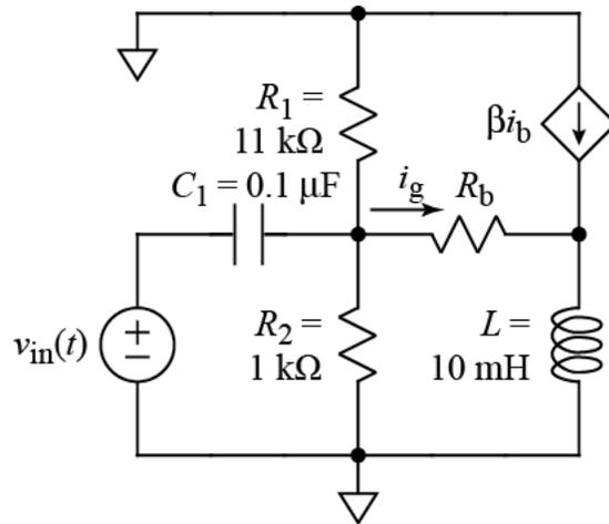
**Note:**  $v_{in}(t) = 300 \cos(800t) \text{ mV}$
