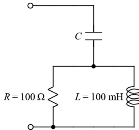
Given  $\omega = 7 \text{ k rad/s}$ , Find the value of  $C$  that makes the total impedance of the above circuit real. You may round off the value of  $C$  to the nearest standard value.
