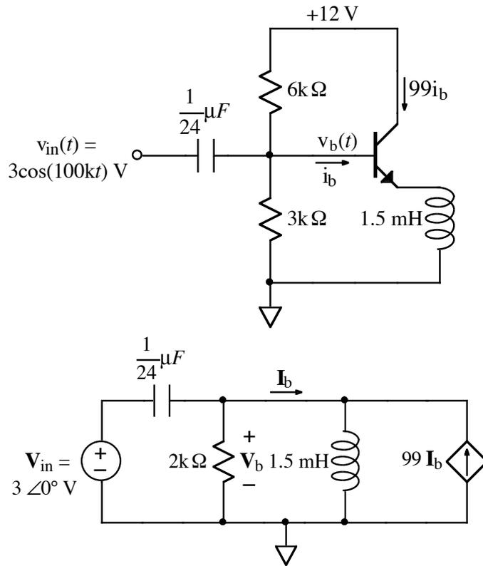
The above circuit diagrams show an emitter-follower amplifier and its high-frequency equivalent circuit. Find  $v_b(t)$ .
