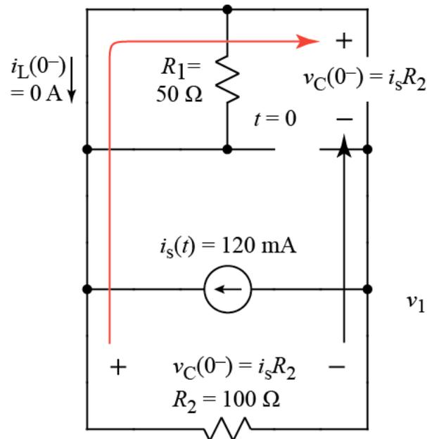
Because of the open circuits, no current can flow in the  $L$ , so  $i_L = 0 \text{ A}$ . As indicated by the arrows in the above diagram, the voltage drop across  $C$  is the same as the voltage drop across  $R_2$ , which is  $i_s R_2$ .
