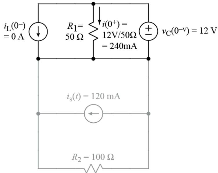
Since the voltage of the capacitor is directly across  $R_1$ , we use Ohm's law to find the initial value of  $i(0^+)$ .
