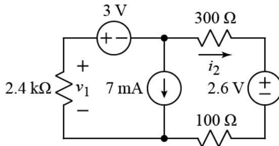
Using the passive sign convention, complete the labeling of all currents and voltages for the resistors in the above circuit.
