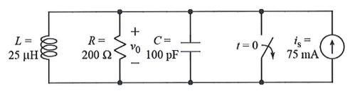
After being closed for a long time, the switch opens at t = 0.
