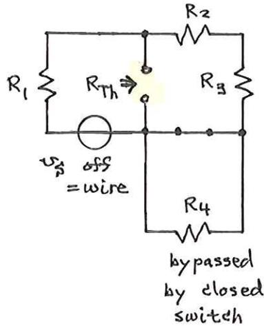
$R_1$  is in parallel with  $R_2 + R_3$ .
