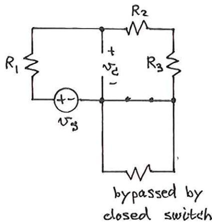
$v_c$  is across  $R_2 + R_3$  in a  $v$ -divider
