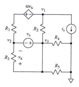
For the circuit shown, write (but do not solve) three independent equations for the node voltages  $v_1$ ,  $v_2$ , and  $v_3$ . The quantity  $v_x$  must not appear in the equations.
