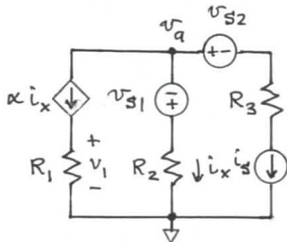
$$\text{Eq'n for node } v_a: \alpha i_x + \frac{v_a + v_{S1}}{R_2} + i_s = 0 \text{ A}$$
