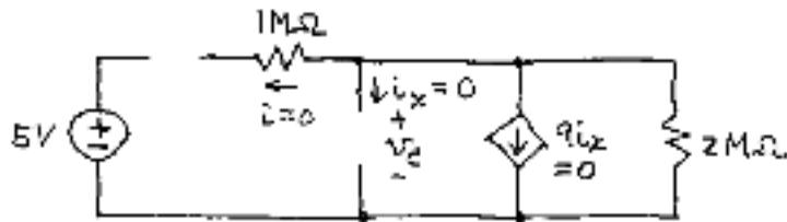
The total current flowing out of top node equals zero, and there is no current flowing in the  $1\text{ M}\Omega$ , the  $C$ , and the dependent source. It follows that the current in the  $2\text{ M}\Omega$  is 0A. By Ohm's law, the voltage drop across the  $2\text{ M}\Omega$  is  $0 \cdot 2\text{ M}\Omega = 0\text{V}$ . This is also the voltage across the  $C$ .
