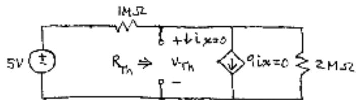
Because there is a dependent source, we find  $R_{Th}$  from  $R_{Th} = \frac{V_{Th}}{i_x}$ .
