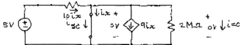
If we short out the output terminals, we have 0V across the  $2M\Omega$  resistor. Thus, there is no current in the  $2M\Omega$   $R$ .
