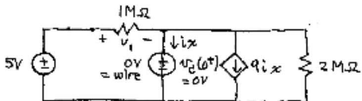
From a voltage loop on the left side, we have  $v_C(0^+) = 5V$ . Note: the components to the right of C are in parallel with the circuitry on the left and directly across the same voltage source, (namely 0V).
