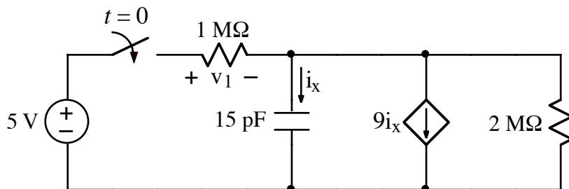
After being open for a long time, the switch closes at  $t = 0$ . Find  $v_1(t)$  for  $t > 0$ .
