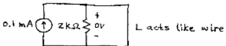
Since the  $2\text{k}\Omega$  resistor is shorted out, it has  $0\text{V}$  across, meaning that the current in the  $2\text{k}\Omega$  is  $0\text{V}/2\text{k}\Omega = 0\text{A}$ .
