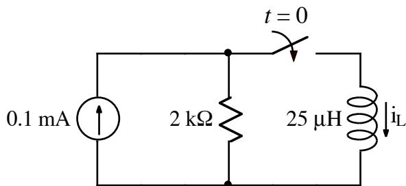
After being open for a long time, the switch closes at  $t = 0$ .  $i_L(t = 0^-) = 0A$ . Find  $i_L(t)$  for  $t > 0$ .
