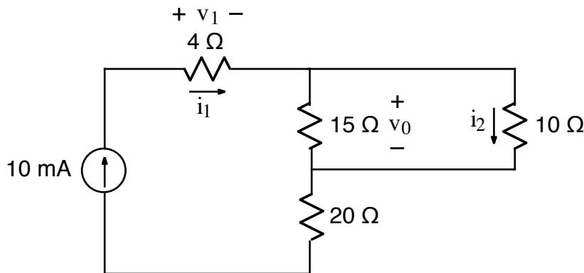
Calculate  $i_1$ ,  $i_2$ , and  $v_0$ .
