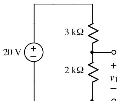
b) Use the voltage-divider formula to calculate  $v_1$ .
