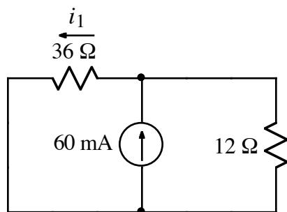
a) Use the current-divider formula to calculate  $i_1$ .
