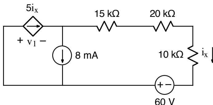
Find  $i_x$ ,  $v_1$ , and the power dissipated by the dependent source.
