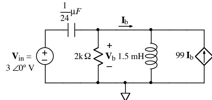
The above circuit diagrams show an emitter-follower amplifier and its high-frequency equivalent circuit. Find  $v_b(t)$ .
