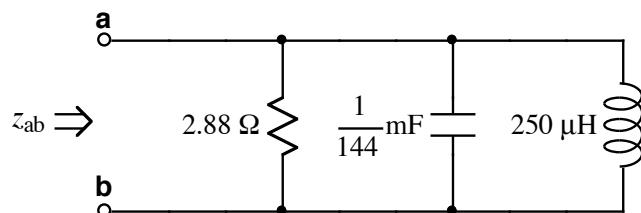
Find a frequency,  $\omega$ , that causes  $z_{ab}$  to have a phase angle of  $-45^\circ$ , (i.e., imaginary part is the negative of the real part). Hint: use admittance, (the reciprocal of impedance).
