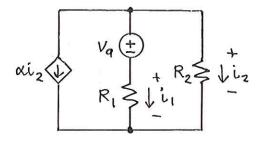
The voltage drops are  $v_1 = i_1 R_1$  and  $v_2 = i_2 R_2$ .
