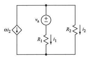
Derive an expression for  $i_1$ . The expression must not contain more than the circuit parameters  $v_a$ ,  $R_1$ ,  $R_2$ , and  $\alpha$ . Note:  $\alpha > 0$ .
