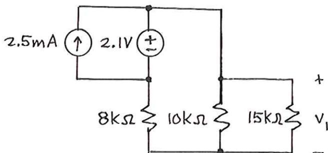
We see that the  $10\text{ k}\Omega$  is in parallel with the  $15\text{ k}\Omega$ .
