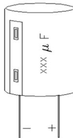
**Fig. 5** Diagram of an electrolytic capacitor with the + and - leads labeled.
