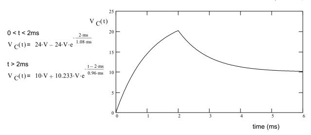
4. For the circuit at right, when is the voltage across R<sub>2</sub> = 10V?
