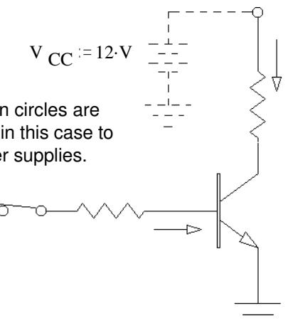
If:  $\beta := 100$        $I_B := \frac{V_{BB} - 0.7\cdot\text{V}}{R_B}$
