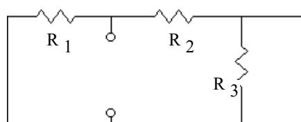
$$R_{Th} := \frac{1}{\frac{1}{R_1} + \frac{1}{R_2 + R_3}}$$
