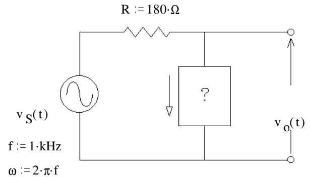
b) Find its value.  $V_o = \frac{\frac{1}{j \cdot \omega \cdot C}}{R + \frac{1}{j \cdot \omega \cdot C}} \cdot V_S$       angle  $\frac{\frac{1}{j \cdot \omega \cdot C}}{R + \frac{1}{j \cdot \omega \cdot C}}$  is  $-90 - \text{atan}\left(-\frac{1}{\omega \cdot C \cdot R}\right) = -90 - \text{atan}\left(-\frac{1}{\omega \cdot C \cdot R}\right)$
