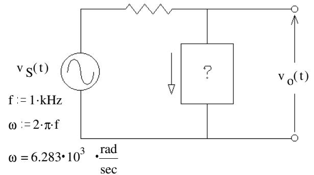
b) Find its value.  $V_o = V_o = \frac{j \cdot \omega \cdot L}{R + j \cdot \omega \cdot L} \cdot V_S$       angle  $\frac{j \cdot \omega \cdot L}{R + j \cdot \omega \cdot L}$  is  $90 - \text{atan}\left(\frac{\omega \cdot L}{R}\right) = 40^\circ$ .
