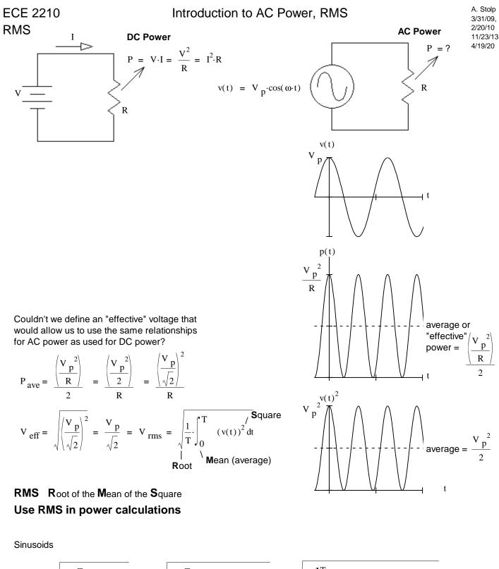
$$V_{\text{rms}} = \sqrt{\frac{1}{T}} \int_{0}^{T} (v(t))^{2} dt = \sqrt{\frac{1}{T}} \int_{0}^{T} (V_{p} \cdot \cos(\omega \cdot t))^{2} dt = \sqrt{\frac{1}{T}} \int_{0}^{T} V_{p}^{2} \cdot \left(\frac{1}{2} + \frac{1}{2} \cdot \cos(2 \cdot \omega \cdot t)\right) dt$$
