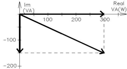
g) The 3 components of the load are in a box which cannot be opened. Add another component to the circuit above which can correct the power factor (make  $\text{pf} = 1$ ). Show the correct component in the correct place and find its value. This component should not affect the real power consumption of the load.
