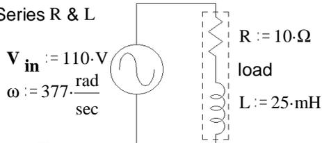
$$Z := R + j \cdot \omega L \quad Z = 10 + 9.425j \cdot \Omega \quad |Z| = 13.742 \cdot \Omega \quad \theta := \arg(Z) \quad \theta = 43.304 \cdot \text{deg} \quad \text{pf} := \cos(\theta) \quad \text{pf} = 0.728$$
