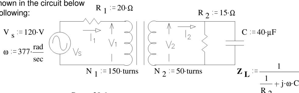
Make an equivalent circuit:
