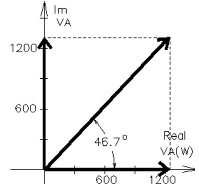
$$\frac{1}{|X_C| \cdot \omega} = 281 \cdot \mu F \quad \text{OR..} \quad \omega = \frac{1}{\sqrt{L \cdot C}} \quad C := \frac{1}{L \cdot \omega^2} \quad C = 281 \cdot \mu F$$
