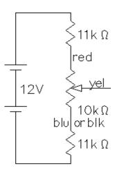
Measure the voltage between the two outside leads of the "Input Position" pot. Turn the pot through its range. Does this voltage change significantly? Now measure from the blue (or black) to the yellow lead and try it again. What range of voltages do you measure?
