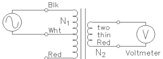
Connect a voltmeter to the secondary
