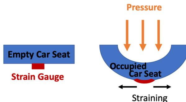
**Fig. 9** A diagram of a strain gauge under a car seat (which could also be built into the car seat). On the left, there is no one sitting in the seat, so there is no strain on the strain gauge. On the right, the seat is occupied, which places pressure on the strain gauge.
