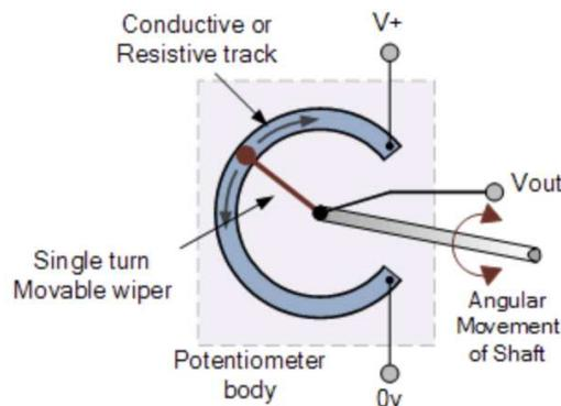
**Fig. 2.** A potentiometer arranged to provide position information (courtesy of electronics-tutorials.ws)
