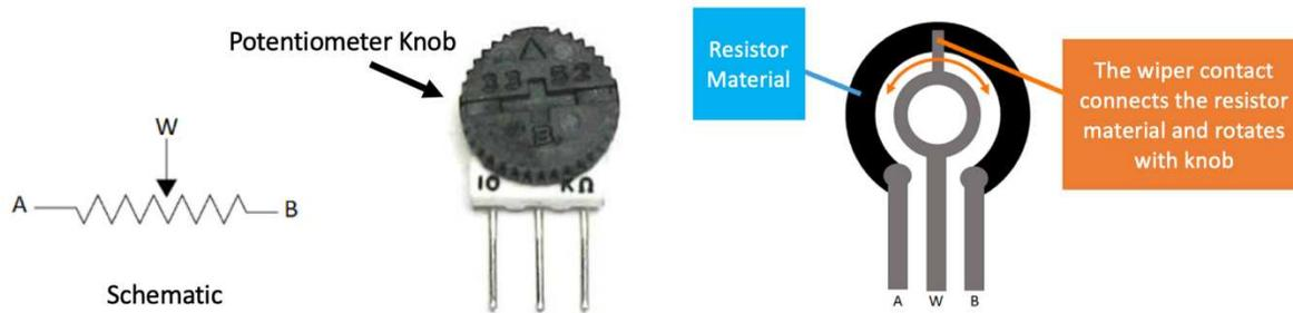
**Fig. 1** A schematic (left side), image (center), and diagram (right side) of a potentiometer (courtesy of Seattle University).
