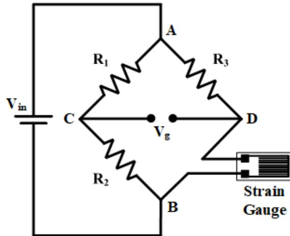
**Fig. 7** A Wheatstone bridge with one strain gauge to measure one unknown resistance developed by the strain gauge (courtesy of hardwarebee.com).
