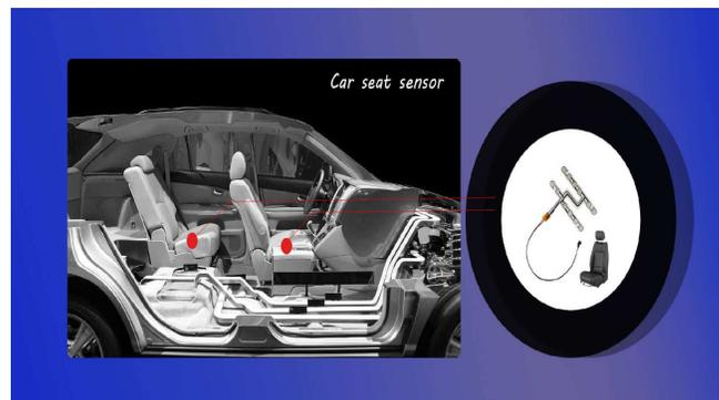
**Fig. 8** Each car seat in a car has a sensor to determine whether someone is sitting in the seat and the weight of that person, i.e. is it an adult or a child, etc. (courtesy of fsrtek.com).
