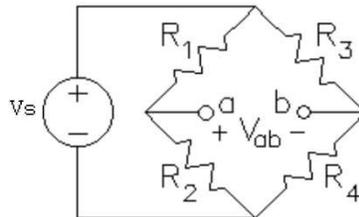
**Fig. 10** The circuit diagram of the Wheatstone Bridge circuit we will build in this lab, with  $R_1$ ,  $R_2$ , and  $R_3$  representing known resistance values and  $R_4$  an unknown resistance (developed from a strain gauge as shown in Fig. 7).
