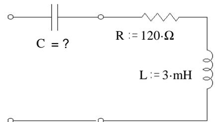
2. You need to design a circuit in which the current  $i(t)$  leads the voltage  $v_S(t)$  by  $36^\circ$  of phase.
