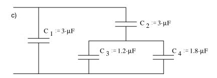
2. Each of the following circuits have been connected as shown for a long time. Find the voltage across each capacitor and the energy stored in each.
