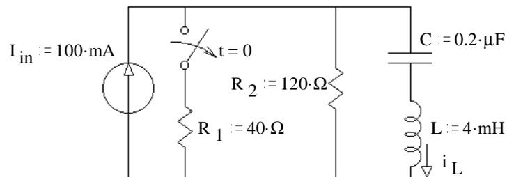
b) Is this circuit over, under, or critically damped?
