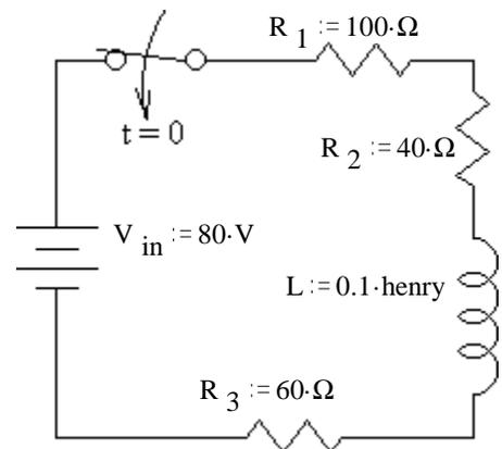
4. In the circuit shown, the switch is closed on position 1 at  $t = 0$ , and then instantly moved to position 2 after 2 milliseconds. Find the time at which the current is zero and reversing its direction.
