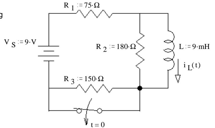
b) Find  $i_L$  at time  $t = 1.2\tau$ .  $i_L(1.2\tau) = ?$   $120\text{mA} - 80\text{mA} \cdot e^{-1.2} = 95.9\text{mA}$
