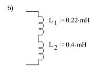
2. Find the stored energy in each capacitor and/or inductor under steady-state conditions. Note: Treat caps as opens and inductors as shorts to find DC voltages and currents.
