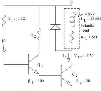
b)  $Q_1$  is in saturation, what is the value of  $R_2$ ? You may assume that the emitter current of  $Q_1$  is approximately equal to the collector current of  $Q_1$ .  $R_2 = ?$
