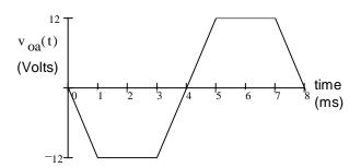
b) Design a circuit which will output the waveform at right.
