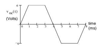
d) Design a circuit which will output the waveform at right. Hint: Think differentiation.
