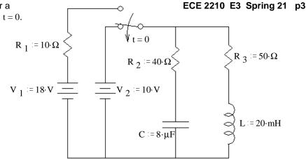
b) Find the initial condition and initial slope of  $i_L$  that you would need to have in order to find all the constants in  $i_L(t)$ . Don't find  $i_L(t)$  or it's constants, just the initial conditions.
