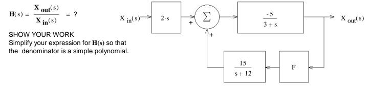
b) Find the value of F to make the transfer function critically damped.
