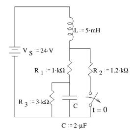
b) Find the initial condition and initial slope of  $i_L$  that you would need to have in order to find all the constants in  $i_L(t)$ . Don't find  $i_L(t)$  or it's constants, just the initial conditions.
