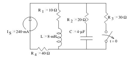
b) Find the initial condition and initial slope of  $i_L$  that you would need to have in order to find all the constants in  $i_L(t)$ . Don't find  $i_L(t)$  or it's constants, just the initial conditions.
