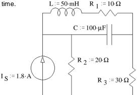
2. (30 pts) The switch has been closed for a long time and is opened (as shown) at time t=0.
