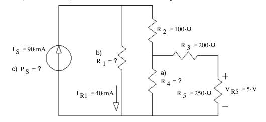
2. (25 pts) a) Use the method of superposition to find  $I_{R1}$  and  $V_{R2}$ . Be sure to clearly show and **circle** your intermediate results.
