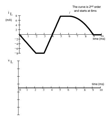
4. The voltage across a 0.5 mH inductor is shown below. Make an accurate drawing of the inductor current. Label your graph. Assume the initial current is 0 mA.
