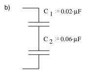
2. Each of the following circuits have been connected as shown for a long time. Find the voltage across each capacitor and the energy stored in each.
